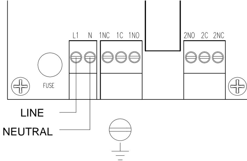
The FDC1000 control unit is powered from 120VAC 50/60Hz at 5VA. Wiring to the unit must comply with the National Electrical Code and local codes. A DPDT relay provides dry contacts for operation of auxiliary alarms or controls at the users discretion. These contacts are rated for 5A at 240VAC or 30VDC.
